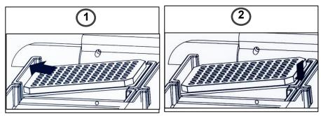
As shown in the picture above, snap the microplate into the heating platform. After installation, it is recommended to press the surface of the microplate vertically and gently to ensure that the installation between the plate and the heating platform is smooth and there is no looseness.
