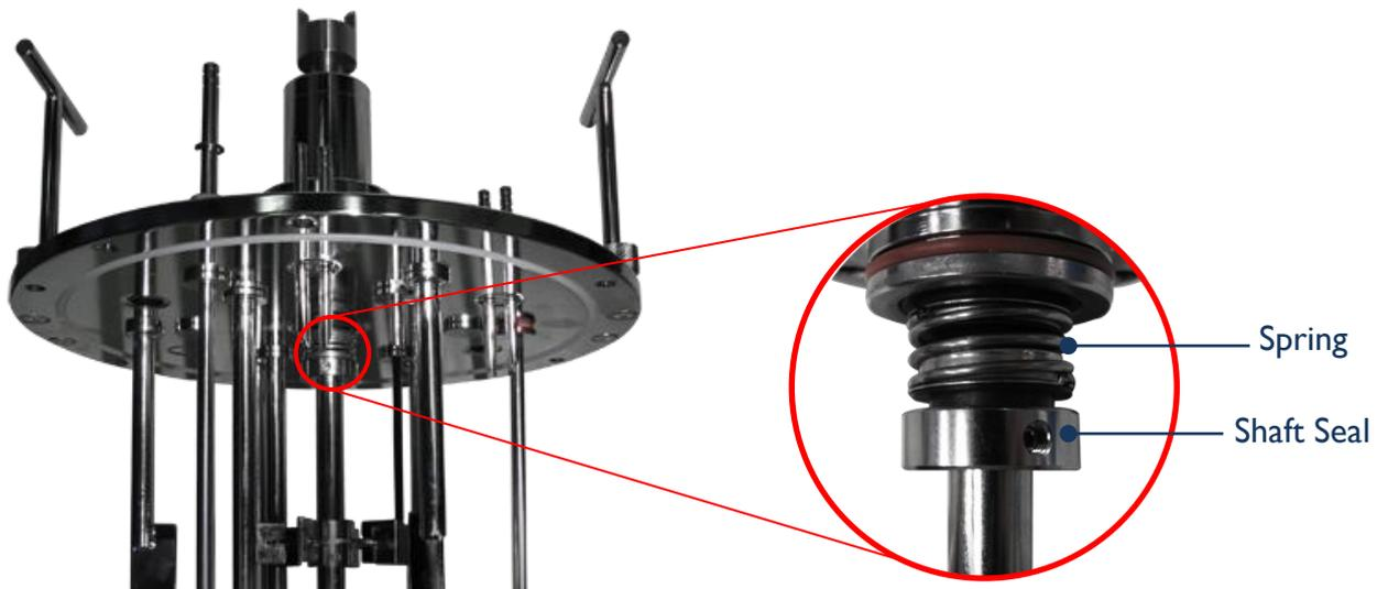
2. Use a small soft brush, such as toothbrush, to gently clean the surfaces of shaft seal and spring with tap water. Rotate the shaft while brushing the shaft seal and spring to make sure the whole surfaces of shaft seal and spring.
