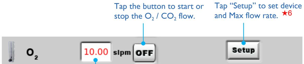
Tap the button to start or stop the O<sub>2</sub> / CO<sub>2</sub> flow.
