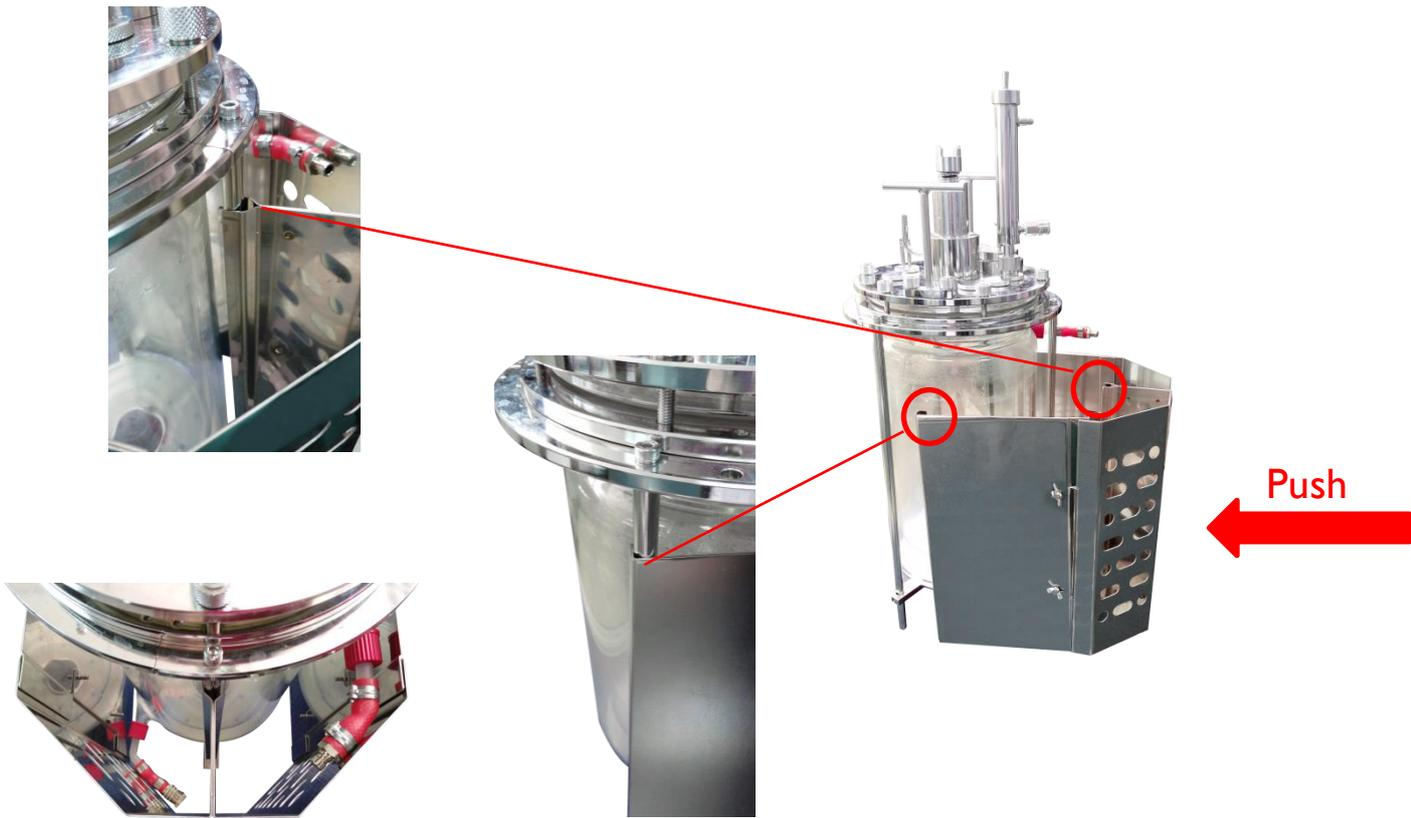
6.3 Tighten the four screws on the protective shield.
