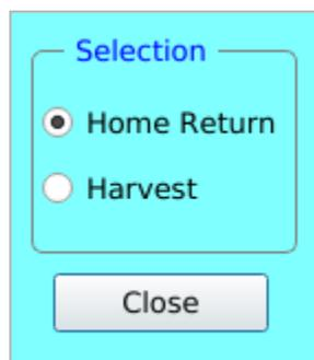
“Home Return” indicates “0 degree” of vessel, if user select “Home Return” then press ”ON”, system would change the angle of vessel to 0 degree; while if user select “Harvest” then press “ON”, system would change the angle to 120 degrees from its previous angle.
