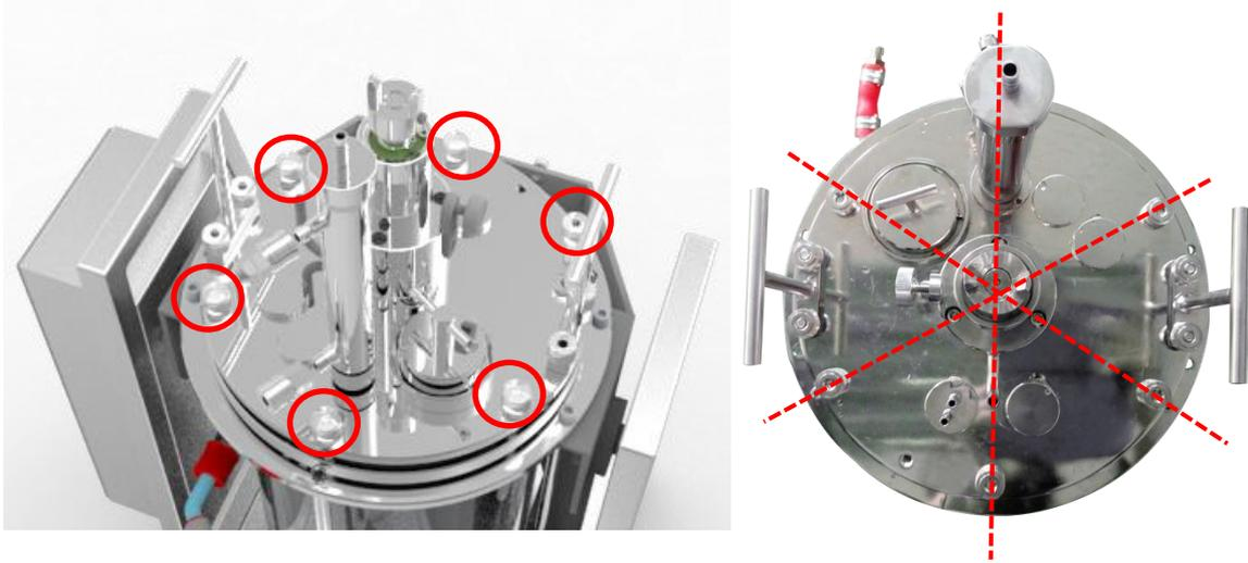
2. Lift up and remove the headplate carefully. Align the screw holes of fixed baffle with the studs, and then lay down two fixed baffles. The slot side face down.
