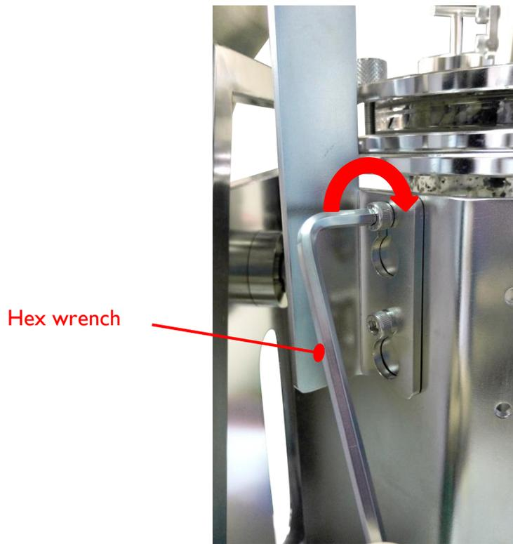
d. Plug in and fix the motor by tightening the screw.
