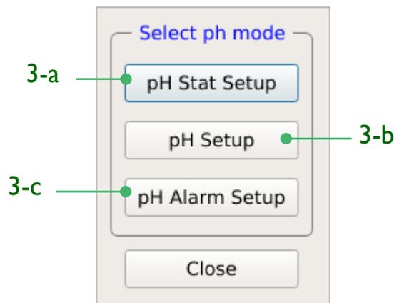
Use “pH Stat” to switch on/off a feeding schedule to a user-defined pH range; pH Setup executes PID control to maintain a pH setpoint. As for “pH Alarm”, user can set up the alarm to alert user when pH value deviates from fluctuations.
