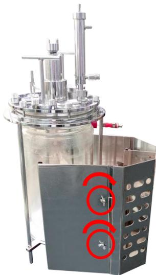
6.2 Align and clip on the three vessel supporters with the protective shield.
