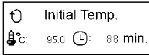
When running Annealing Program Mode, the current temperature of block and the step settings will show on the screen
