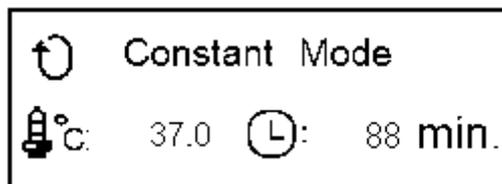
When running Constant Mode, the current temperature of block and the step settings will show on the screen.
