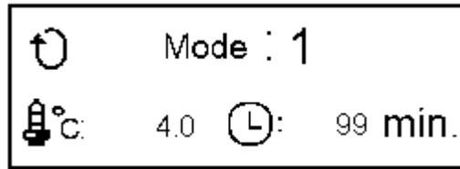
When running Quick Start Mode, the current temperature of block and the step settings will show on the screen.
