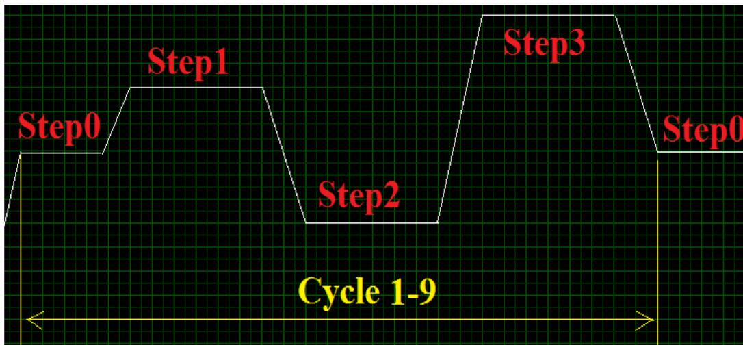
**Annealing Program:** There are setting parameters for Initial Temp., Descending Temp., Holding Time, and Final Temp.
