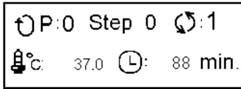
When running Programmable Mode, the current temperature of block and the step settings will show on the screen.
