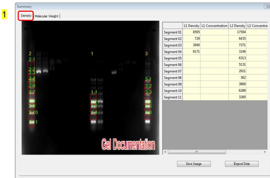
**Step2** Double click the blank L1 Concentration box associated with the known marker size. After key in the first value, the system will show a dialog to remind you to key in the second value.
