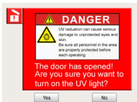
If the UV transilluminator is on while the door is opened, UV light will be turned off automatically, and the warning will pop up to warn users that the UV light is harmful to humans if protection mechanism is not prepared. Press "Yes" to turn the UV transilluminator on or "No" to cancel turning on the UV transilluminator.
