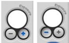
Press “+” or “-” under the column of “Exposure” to increase/decrease 0.001 sec. of the value of exposure user sets.
