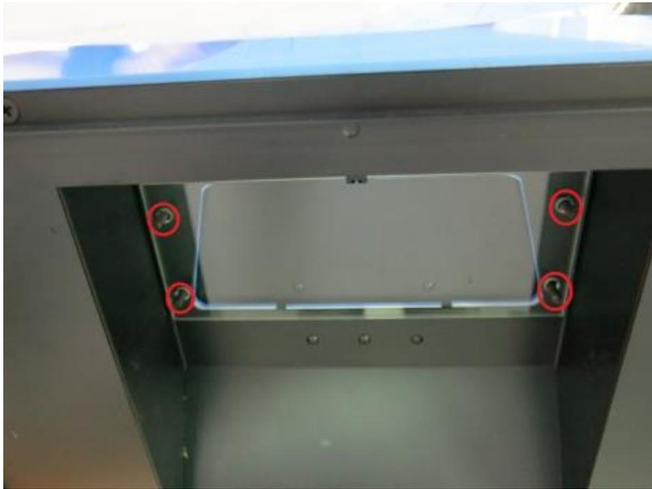
**Step2** There are no screw holes on the amber filter, please put the amber filter in between.
