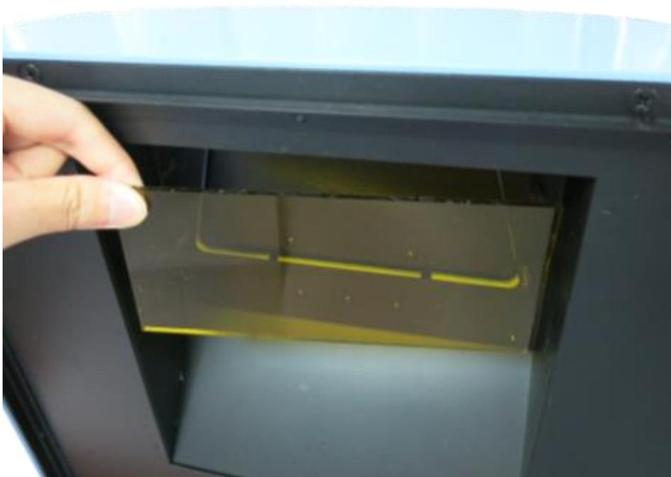
**Step3** Replace the transparent filter, put the nuts of four corners and then use the socket wrench to tighten the nuts.
