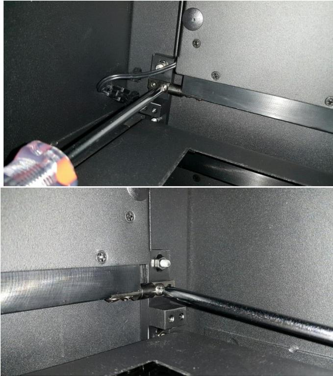
**Step4** Connect the White Light Plate cable to darkroom inner socket.
