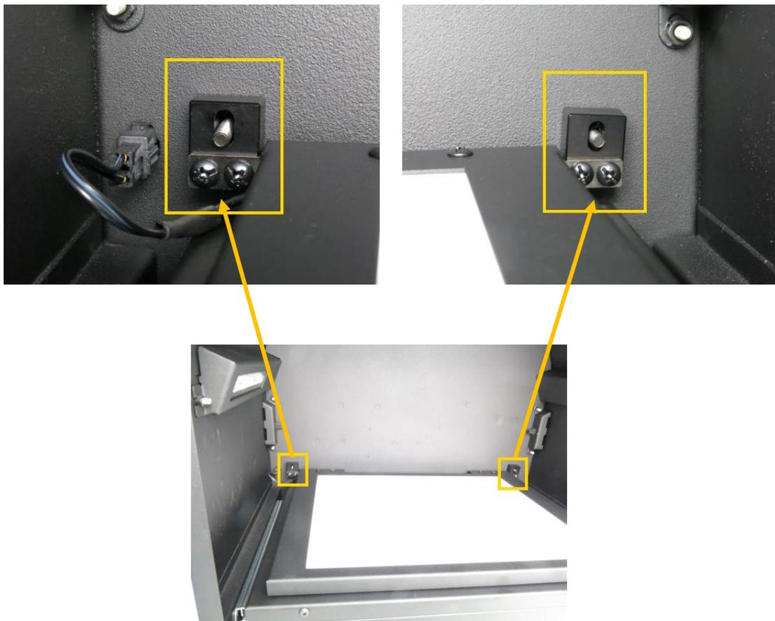
**Step5** To take nuts from parts kit. Use 7M/M socket wrench to tighten nuts on the studs.
