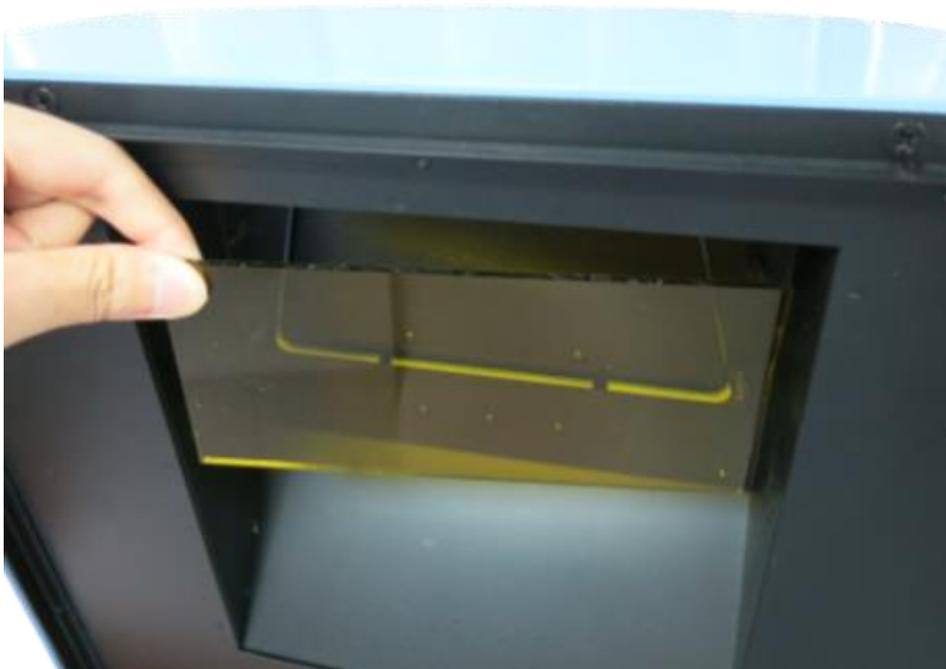
**Step3** Cover the transparent filter on the amber filter, put the nuts of four corners and then use the socket wrench to tighten the nuts.
