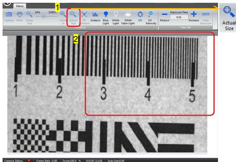
**Step2** Put fluorescent ruler on the UV table again. Turn on the UV light and press “Actual Size” button (as box 1) to make sure the picture is clear and focus on. Fix the focus ring after adjust.
