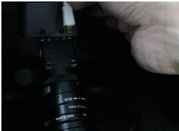
**Step5** Separate the camera with darkroom, you could use general camera cleaning kit to clean the lens and then reinstall the camera on the camera holder for clearer image.
