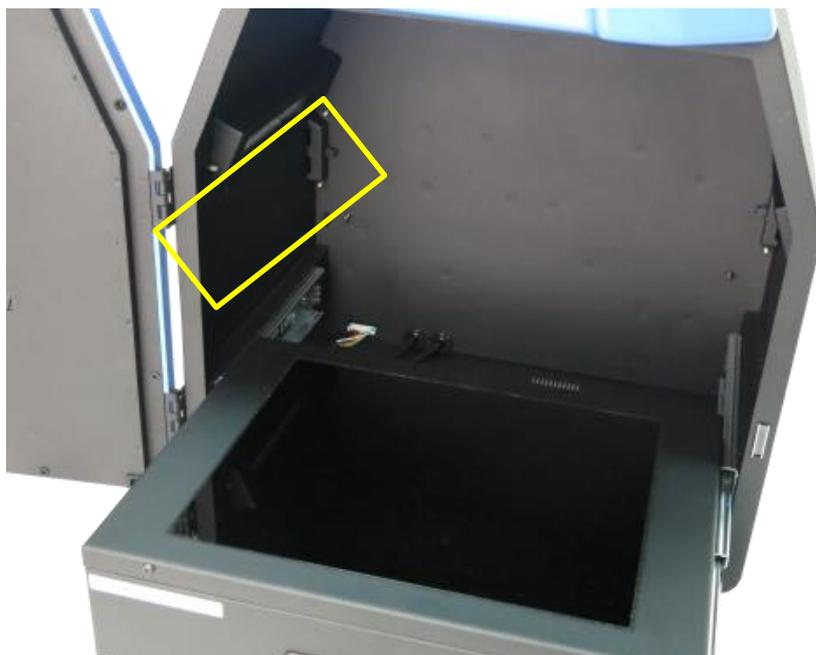
**Step3** Connect the blue light quick connector with darkroom inner socket.
