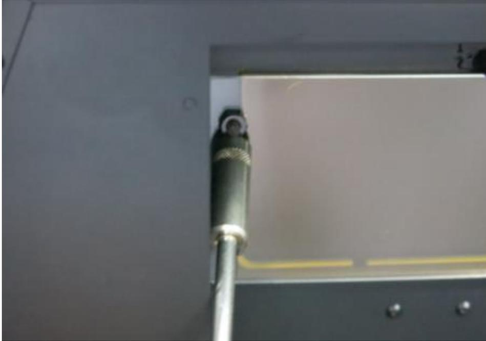
**Step4** Confirm the amber filter is be fixed in the center of the viewing window.
