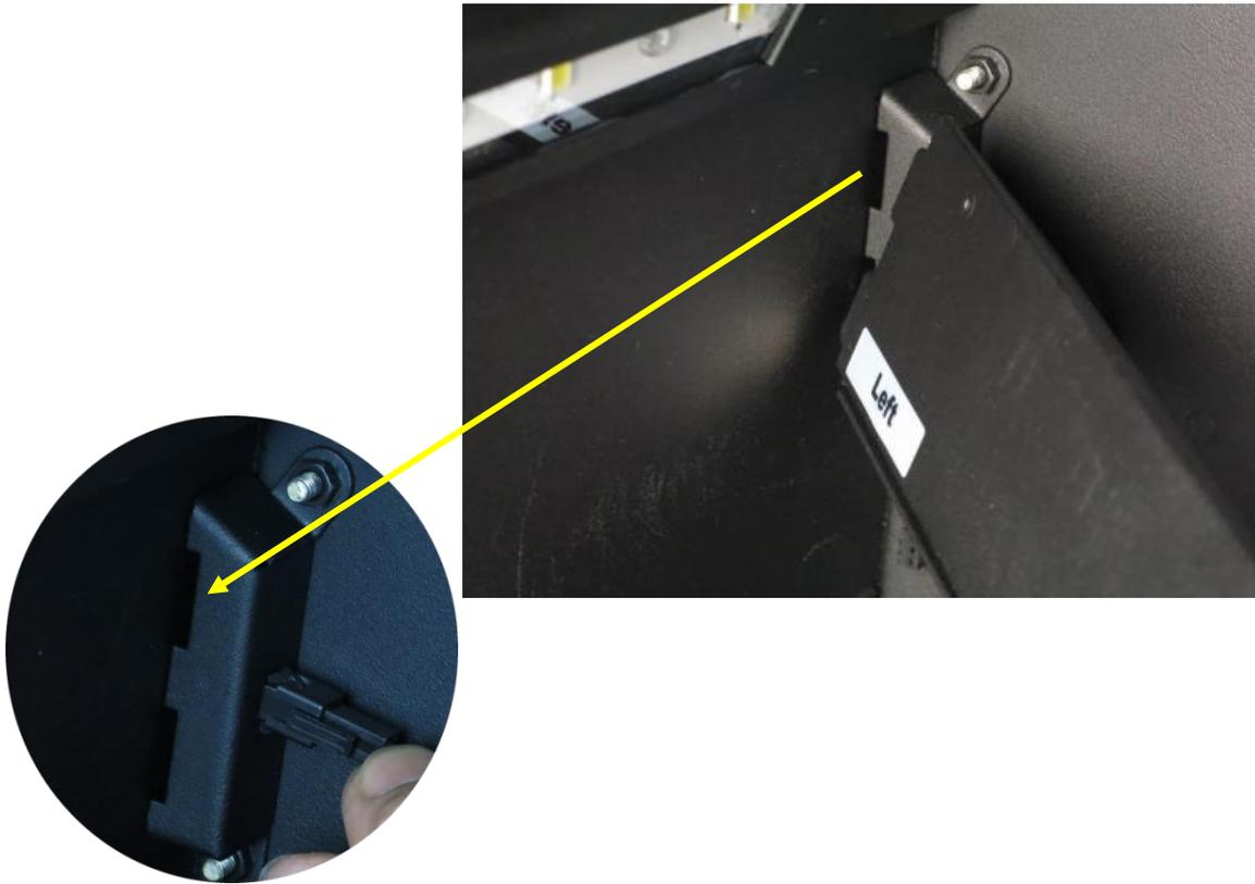
**Step5** Put the other side of blue light into the stud of darkroom inner wall.
