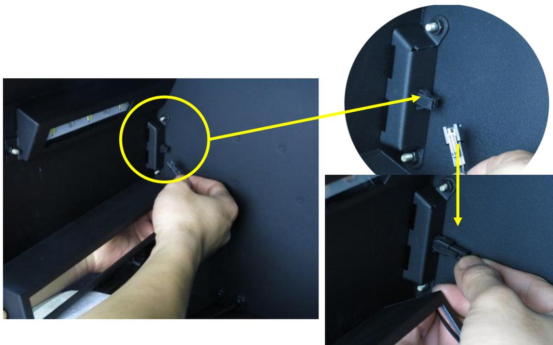
**Step4** Insert the blue light into the inner lining of darkroom.
