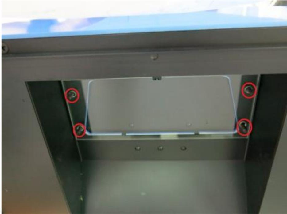
**Step2** There are no screw holes on the amber filter, please put the amber filter on the inside of the bolt.
